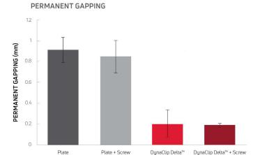
The DynaClip Delta with a crossing screw and DynaClip Delta constructs both demonstrated **4x less permanent plantar gapping** than a plate with a crossing screw and the standard plate constructs after destructive bend testing.<sup>1</sup>
