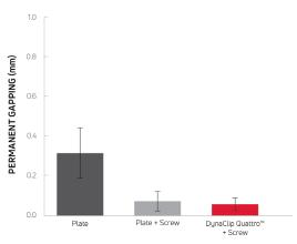
The DynaClip Quattro with crossing screw construct demonstrated 6x less permanent plantar gapping than the plate construct and demonstrated equivalent permanent plantar gapping to the plate with crossing screw construct after cyclic bend testing.<sup>1</sup>
