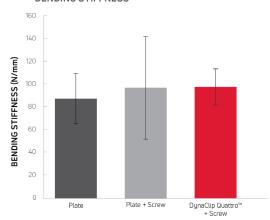
The DynaClip Quattro with a crossing screw construct demonstrated equivalent bending stiffness to both plate with a crossing screw and standard plate constructs.<sup>1</sup>
